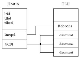
In the following diagram, each host is connected to at least one drive and the robotics are controlled from Host A. ltid on each machine initiates tlhd. The tlhd on Host A also initiates tlhcd, since that is where the robotic control is defined. Requests to mount tapes from Host B go to tlhd on Host B, which sends the robotic command to tlhcd on Host A.
